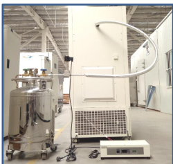
LN 2 /CO 2 backup system
