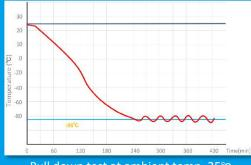
Pull down test at ambient temp. 25°C
