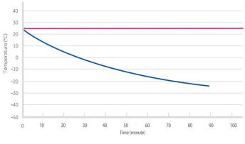
MDF-25V268E Pull Down Test at Ambient
